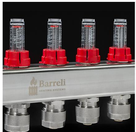
Because the manifold is equipped with flowmeters, the inlet water flow rate for each circuit can be controlled. Consequently, the volume of hot water entering the circuit is adjusted, and the heat output for that specific zone can be regulated.
